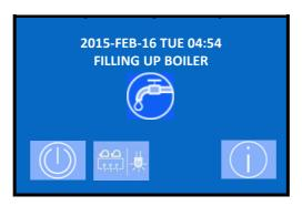
• Afterwards the keypad lights will be off and heating of the boiler starts. Please wait about 15 minutes to reach the set temperature
