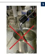
Do not leave the steam wand into any liquid at any time.
