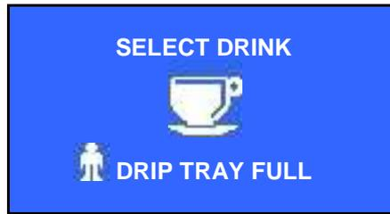
Cause: the drip tray is full, the quantity of water inside the drip tray touches the level probe.
