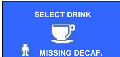
Cause: Missing coffee in the decaffeinated door and in the brewing chamber
