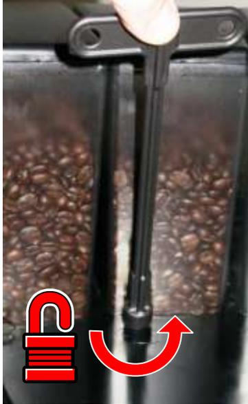
b) Move the adjustment to the right to get coarse coffee powder, to the left for finer.
