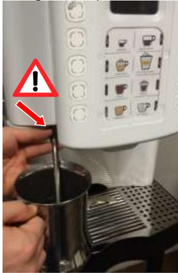
3► Press the steam button to stop the delivery before removing the jug.
