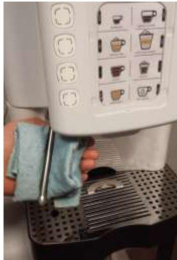
6► **DO NOT** leave the steam wand into any liquid at any time
