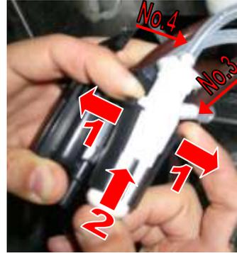
4► Disassemble the milk frother in all its parts (first by turning and then by pulling as shown in the picture) and wash it either by hand or in a dishwasher. Make sure that all the holes are free from milk residues and also to use provided tools to clean the holes. Check also that the O-rings are in good condition
