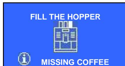
to reset the alarm put coffee into the hopper and press again the dose required.
