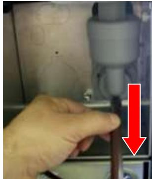
3► Turn the flange 1 anticlockwise, then remove the mixer 2
