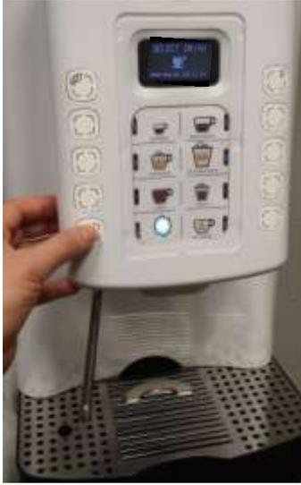
2► Use the steam wand to foam or heat any liquid into the jug by handling the rubber protection.
