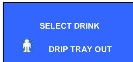
Cause: the drip tray is not in position. The micro switch contact is open.
