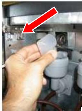
b) Place the provided cap on the canister to avoid that the powder product comes out during disassembly
