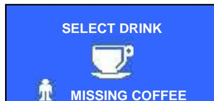
Cause: there is no coffee into the hopper and therefore into the brewing chamber
