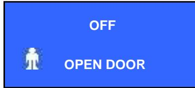
Cause: the front door is open; the micro switch does not touch the door
