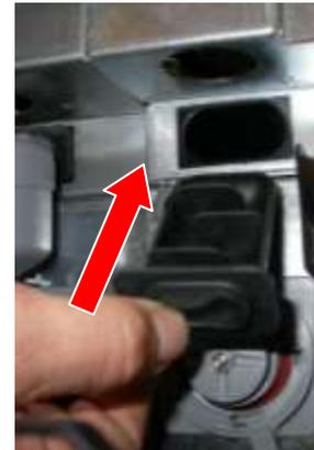
7► Turn the flange clockwise to reinsert the mixer
